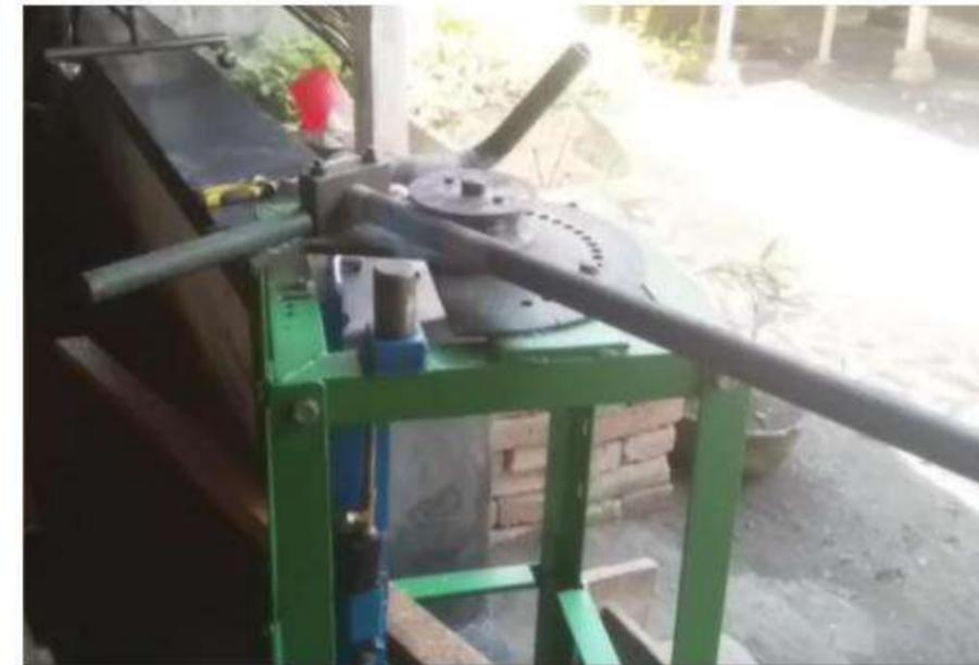
Gambar 5.7 Ujicoba mesin bending
